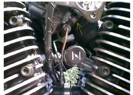
I used a 1/8" bit. The metal is very soft so don't apply much pressure while drilling.
