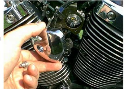
The arrow in this image points to the pilot screw plug for the carb on the right side of the bike. This would normally be hidden by the air cleaner housing.
