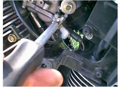
Use a pair of pliers to wiggle the screw up and down and gently pull the plug out.
