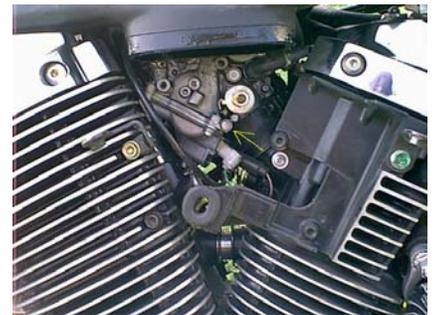
The arrow in this image points to the pilot screw plug for the carb on the left side of the bike.
