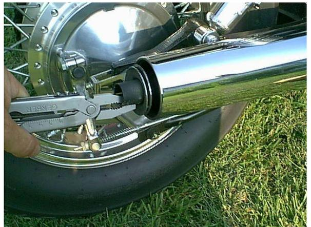
Just wiggle the pliers up and down and side to side while pulling to completely remove the insert from the pipe.
