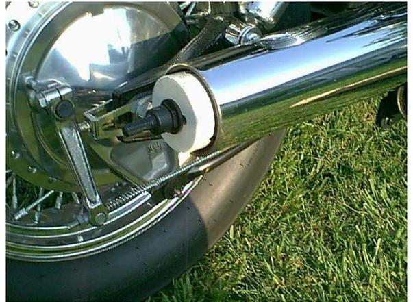
This next image shows that you will have to drill thru 2 pieces of metal before you can remove the insert. You will feel the saw give as it cuts thru the first layer, just keep going until you feel it go thru the second as well. Don't worry about hitting anything you shouldn't because as you will see later there is nothing else in the pipe within reach of the saw. Once you cut thru the second layer you should be able to wiggle the insert with a pair of pliers.
